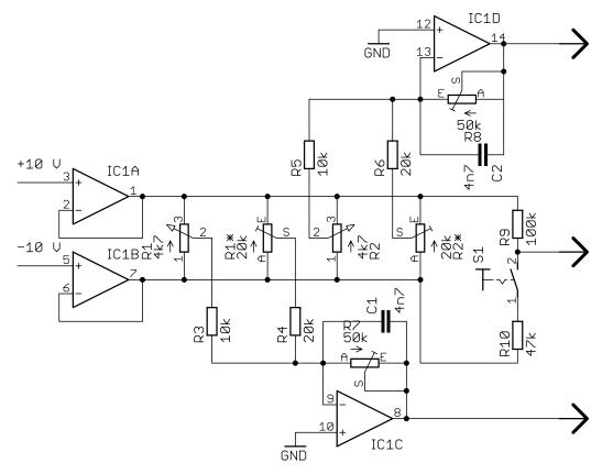
Figure 1: Joystick adapter circuit
