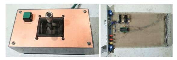
Figure 2: Joystick mounted in enclosure and prototype adapter circuit
