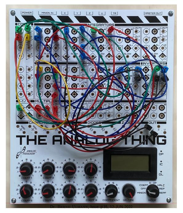
Figure 3: Setup for generating  $J_0(\tau)$  and  $J_1(\tau)$
