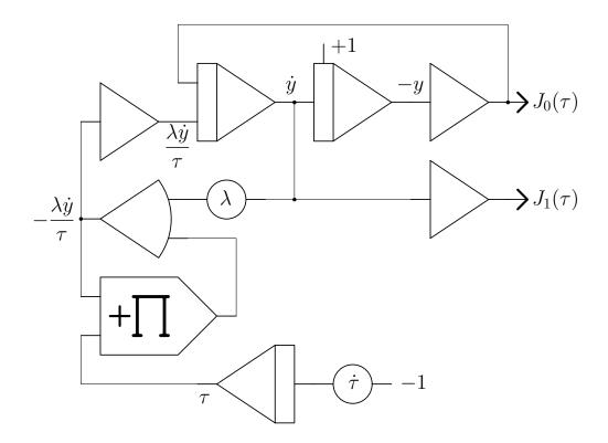
Figure 2: Analog computer program for generating  ${\rm BESSEL}$  functions  $J_0(\tau)$  and  $J_1(\tau)$
