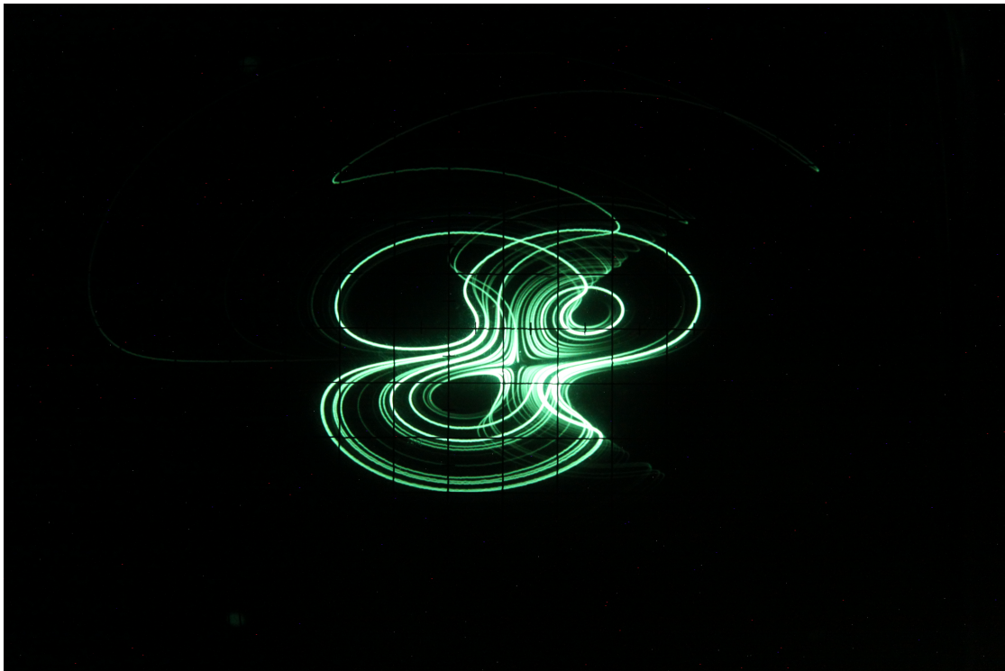
Figure 4: Phase space plot of the DADRAS system with c = 1.7 instead of c = 4.7
