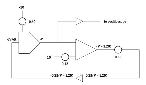
Figure 1: Computer setup for Newton's law of cooling
