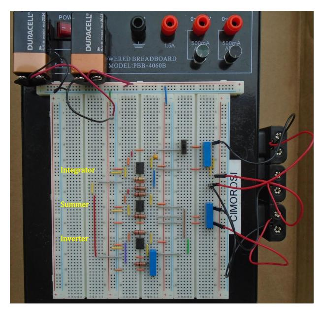
Figure 4: Differential Equation Analog Computer
