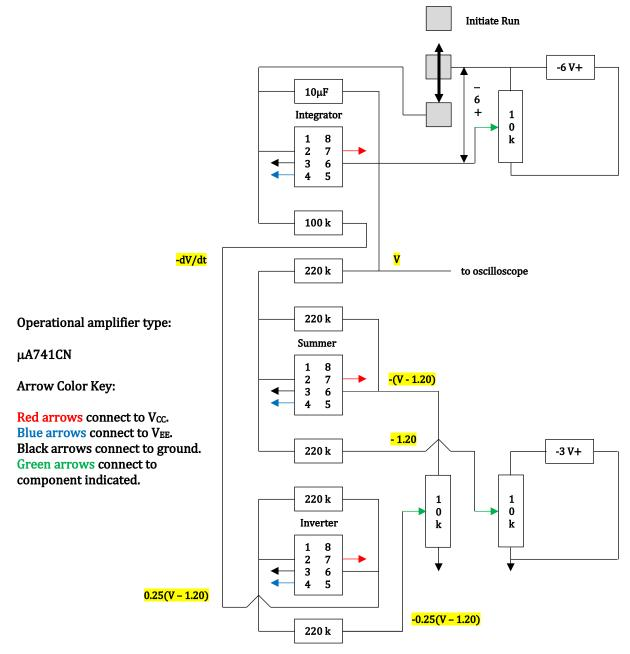
Figure 2: Basic breadboard layout
