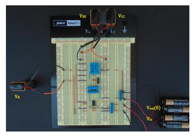
Figure 2: Photograph of inverting integrator breadboard layout
