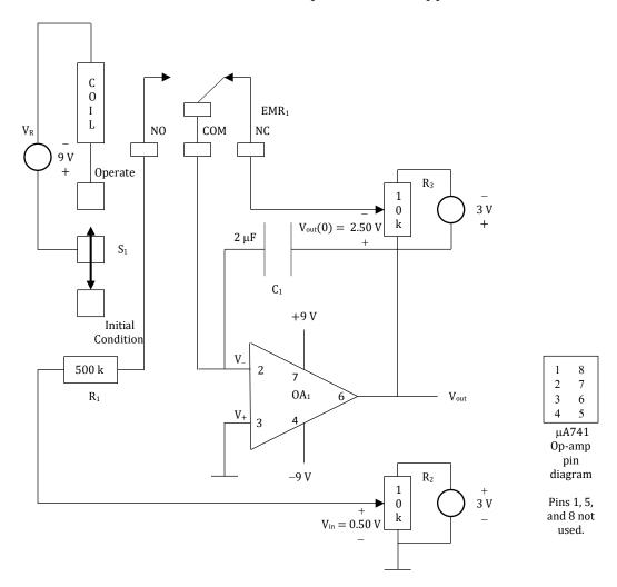
Figure 1: Inverting integrator diagram
